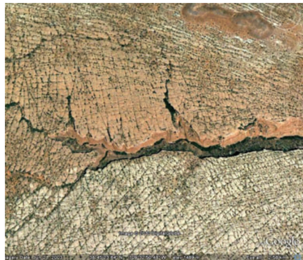
Figure 2 Orthotropic (top) and monoclinic (bottom) symmetries in fractured sandstone, Arches National Monument.
